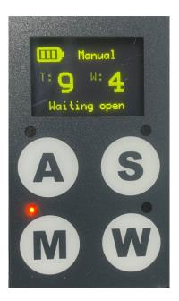
4- Press the opening button to open the tool for insert the strap. On the display appears the written "OPEN".
