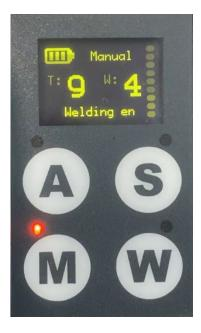
8- At the end of the welding start the countdown (3-2-1), indicating the cooling time, followed by end of cycle sound. When the cooling time is finished, on display appears the written "WAITING OPEN". Press the opening button to open the tool and remove it from the strap. Completed this operation you are ready for another cycle.
