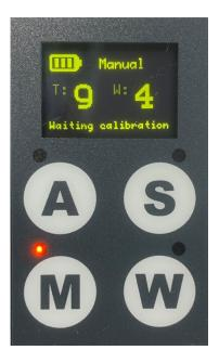
2- Press the opening button to do the calibration of the AUTOMATIC OPEN SYSTEM. On the display appears the written CALIBRATION". This operation must be done every time the tool is turned on or when it enter in sleeping mode (more than 4 hours).
