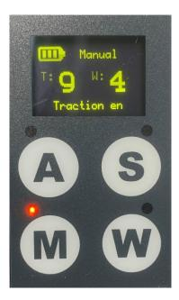
6- Press the tension button and the tool will begin tensioning. On the right of the display appears indicator that show the progress of tensioning highlighting tension reached.
